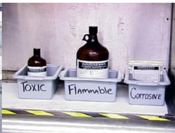
Hazardous waste stored in a Satellite Accumulation Area
