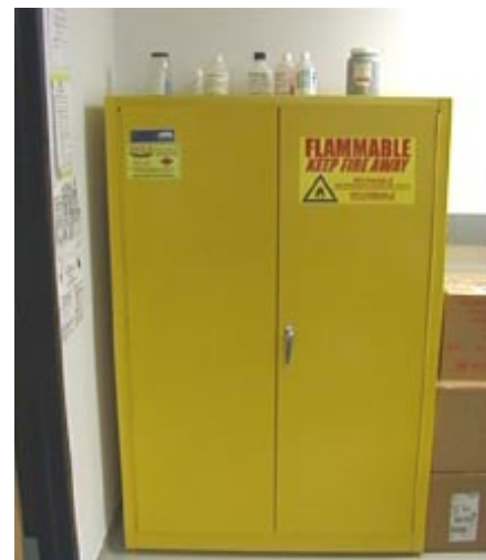
Proper laboratory storage of flammable materials in an approved cabinet.
