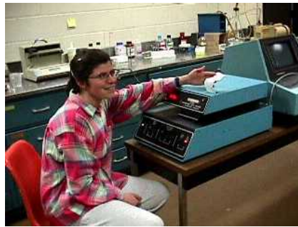
Dynatech ELISA Plate Reader Used for plate readings for immunoassays
