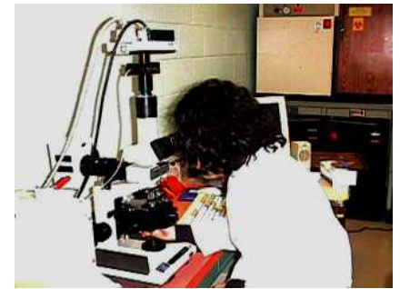
Olympus Fluorescence Microscope Used to analyze GFP (Green Fluorescent Protein) producing bacteria
