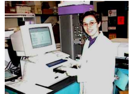
Dynex Mycroplate Reader Used to study chemical or microbiological reaction kinetics.
